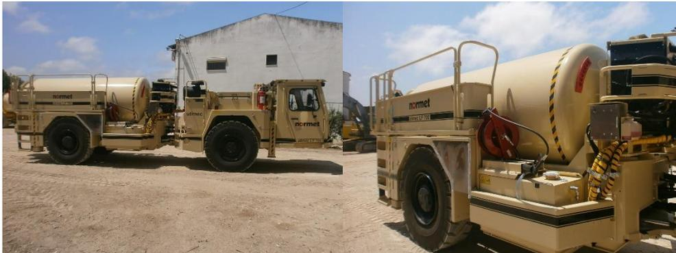
**Figura 2:** Autobetoneira Normet Utimec LF 700 Transmixer HE491.
