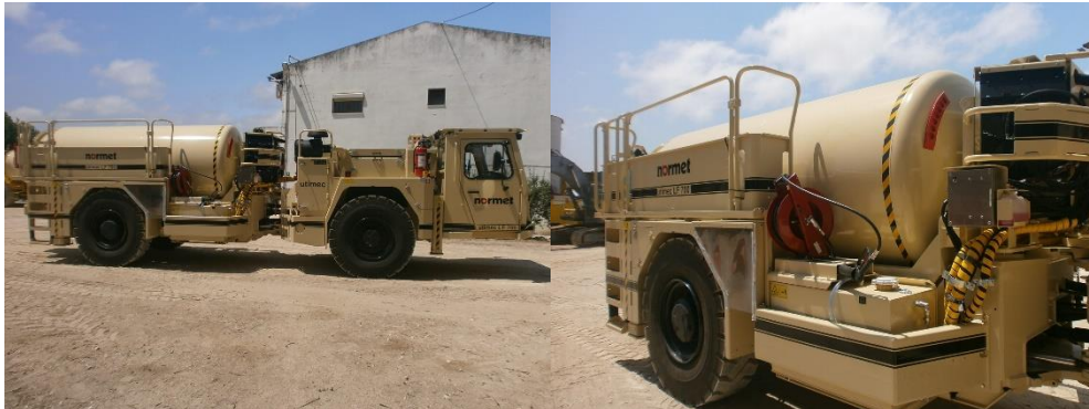
Figura 2: Autobetoneira Normet Utimec LF 700 Transmixer HE491.
